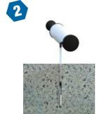
Clean hole with compressed air or vacuum to remove any excess dust/debris.
