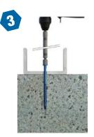
Place XCS setting tool with drive socket over drill bit.
